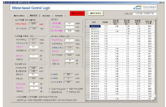
Figure 6. Implementation of a post-chlorination controller.
