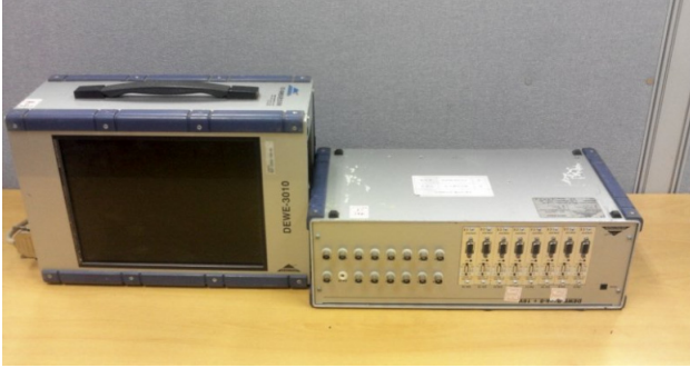
Figure 7. Data acquisition system (DEWE-3010).
