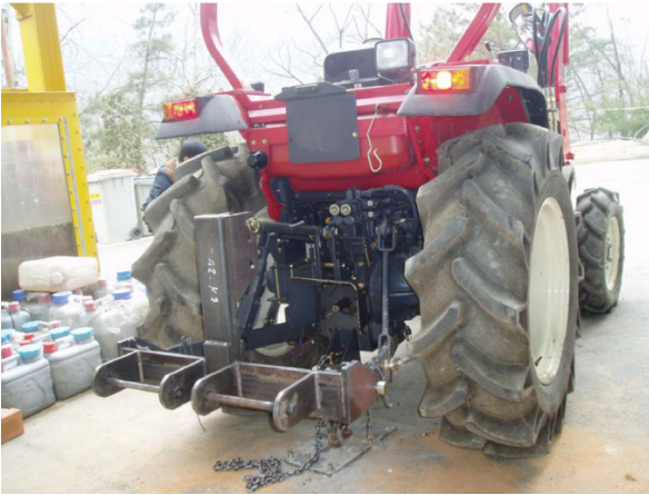
Figure 5. Anchor to connect the tractor to the ground.
