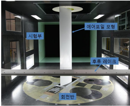
Fig. 2. Test set-up of the airfoil model in the test section
