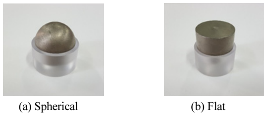
Fig. 2 Configuration of projectile nose shape
