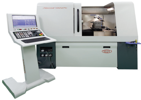
Fig. 1 Ultra-Precision diamond turning machine (Nanotech 450 UPL, Moore technology)
