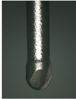
Fig. 2 A CBN end-mill tool for machining the arcs
