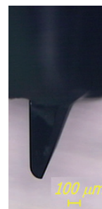
Fig. 7 A diamond end-mill tool for machining of the arcs
