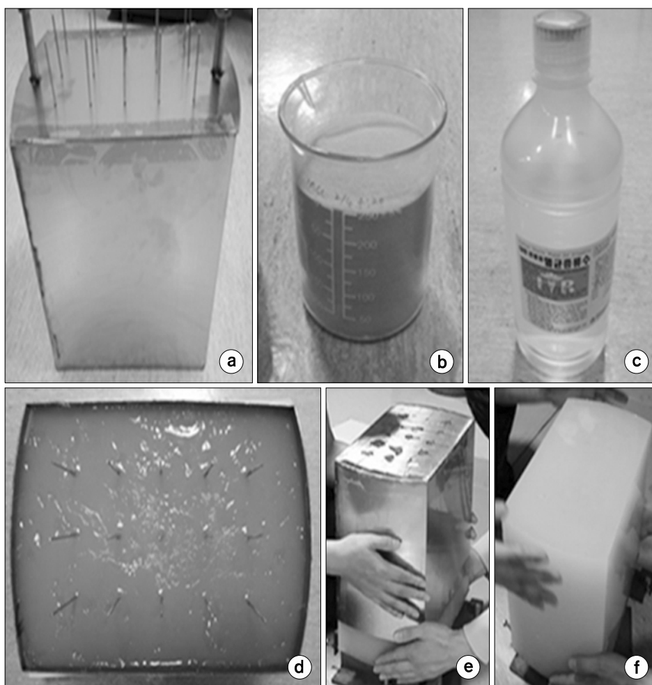
Fig. 1. Making of agar phantom: (a) Agar phantom mold, (b) Agar powder of MSC Co. Ltd, (c) Sterile water, (d) Gel agar solidified with phantom, (e) Gel agar phantom separated from the mold, (f) Completed production of agar phantom.
