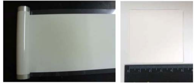
Fig. 4. (a) Green sheet of LLZO on PET film and (b) stacked plate of LLZO with 320 \mu\text{m} in thickness.
