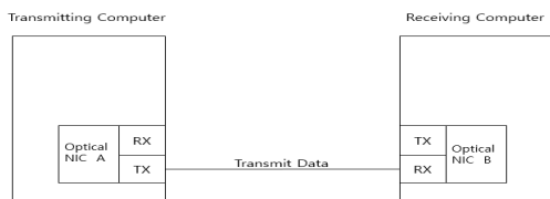
Fig. 3. Unidirectional transmission using modified device driver
