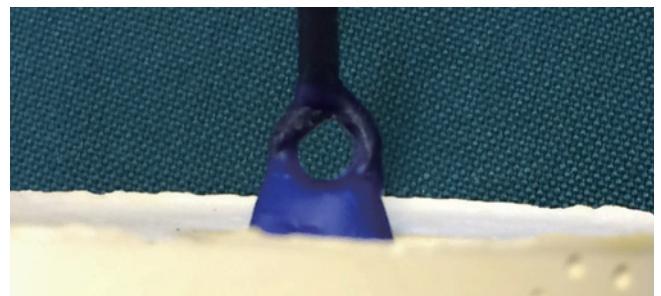
Fig. 2. Wax pattern. A ring was placed on the occlusal surface, sprued, and casted. This ring was used for attachment to the jig of the universal testing machine for tensile strength testing.
