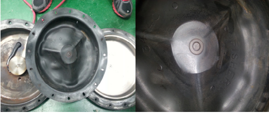
Fig. Photo 9 Nitrile Diaphragm 최종검사(Crack)
