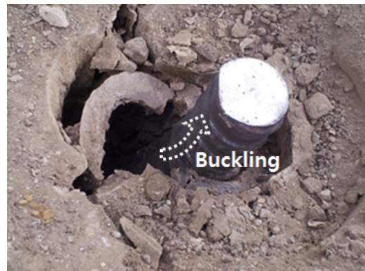
Fig. 9. Buckling shape of reinforcing steel bar
