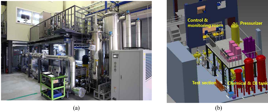
Fig. 1. FAC simulation test facility designed to operate in conditions of 6.0 MPa pressure and 270 °C temperature with maximum flow velocity of 20 m/s for pipe diameter of 2 inch: (a) photo Picture of operating test facility and (b) 3 dimensional layout.
