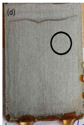
Fig. 18. Optical photograph of 15 % Ch/5 % Gr 2 SiO 2 PVB coatings after 1 week immersion in 0.5 M salt solution.
