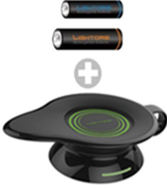
Fig. 1. Concept of the proposed wireless power rechargeable battery charging system.
