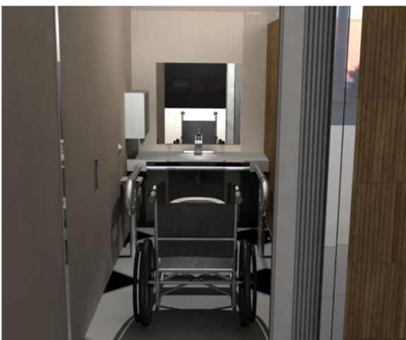
Figure 5. Front-entry sitting restroom system (backside view)
