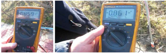
Fig. 12. PS potentials according to the position of reference electrode at T/B A.
