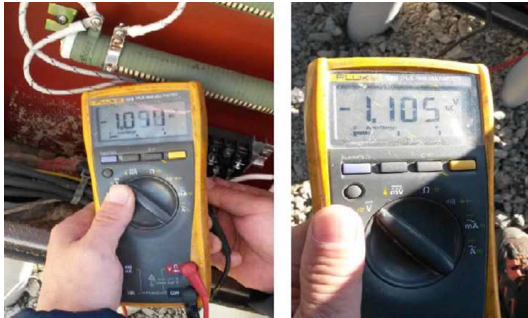
Fig. 13. PS potentials according to the position of reference electrode at T/B B.
