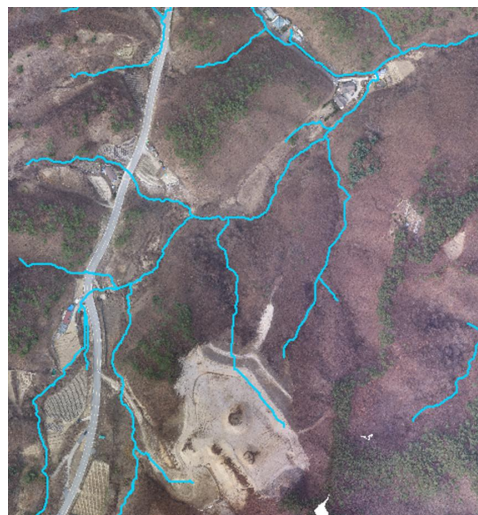
Figure 23. Result of drainage line extraction (after)
