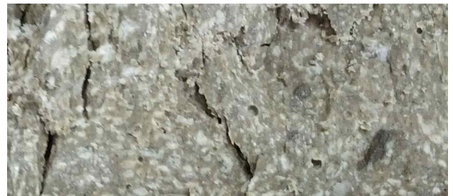
Figure 6. Fracture surface of cement paste with bentonite; white spots are coagulated bentonite particles
