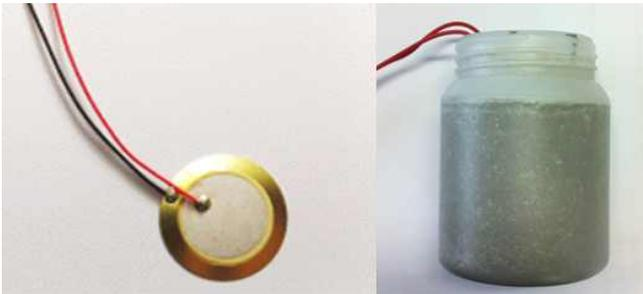
Figure 1. Piezoelectric sensor embedded in cement paste
