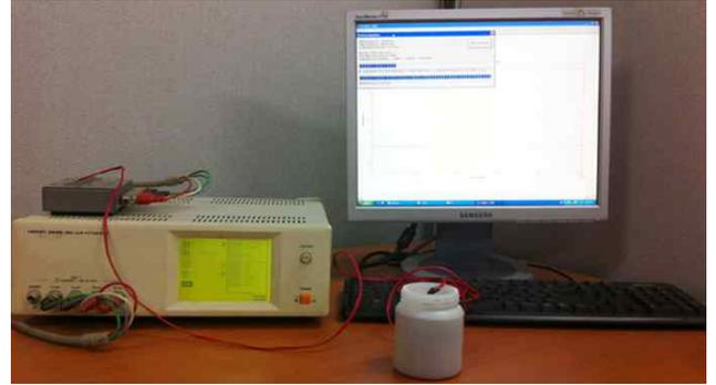
Figure 2. Test setup for measuring EMI of PZT sensor
