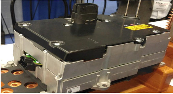
Fig. 7. Volt 2nd generation inverter.
