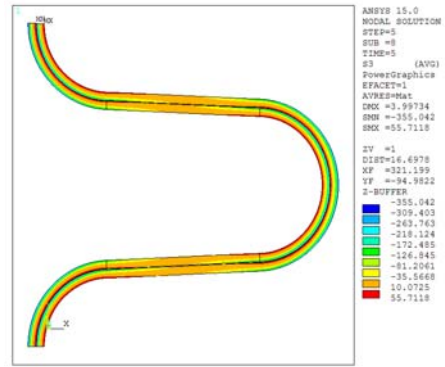
Figure 7: Contour of convolutions stress at displacement 22.0 mm
