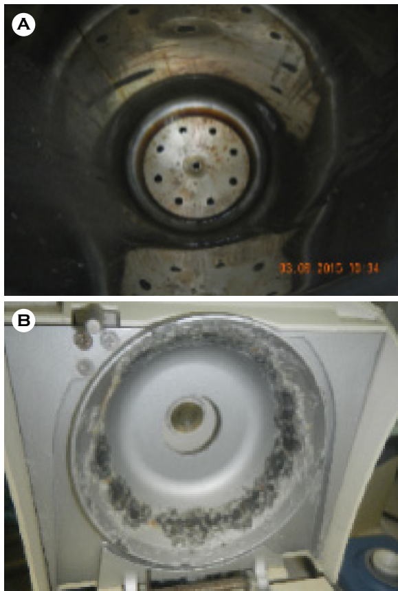
Fig. 4. Poor maintenance of equipment: (A) corroded autoclave with dirty water inside. (B) Corroded and dirty centrifuge cover.
