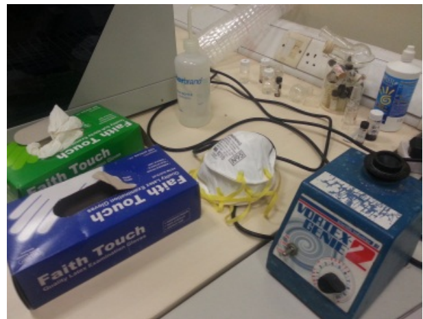
Fig. 5. Used N95 mask was left on the bench together with other contaminated items. It should be disposed of immediately after its use. In case of reusable mask, the mask should be sanitized and sealed in plastic bag and kept away separately.
