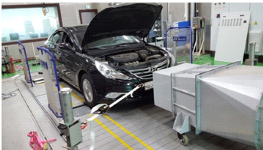
Fig. 2 Photograph of test vehicle on the chassis dynamometer
