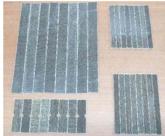
Fig. 3 Configuration of tension and compression in plane-shear, flexure specimen
