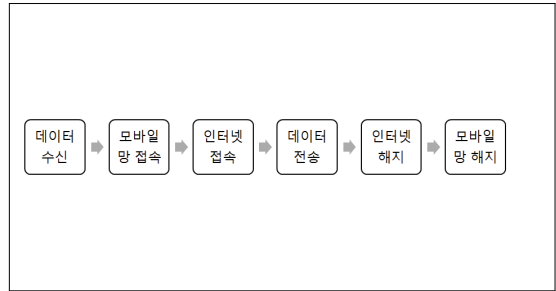
Fig. 2. Network connection process of the gateway
