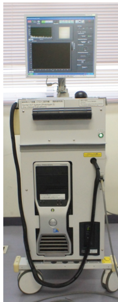
Fig. 2. A photograph of the machine of a dental optical coherence tomography system (Prototype 2; Panasonic Healthcare Co., Ltd., Ehime, Japan).
