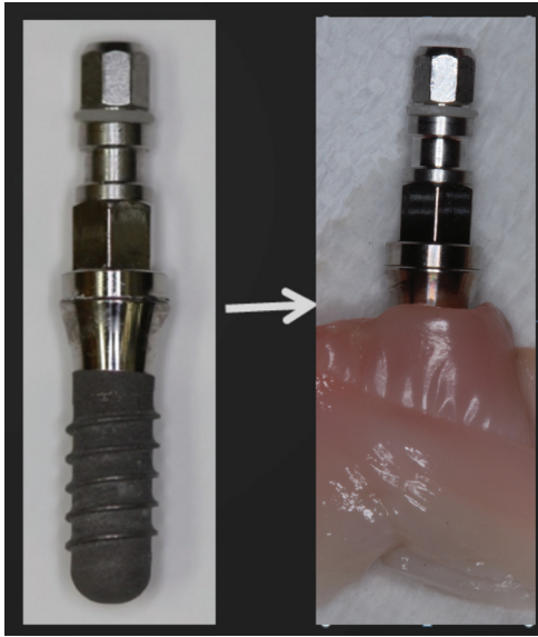
Fig. 3. A dental implant (Straumann standard implant RN) is covered with pig's oral mucosa for evaluating the detectability of an implant underneath mucosa via optical coherence tomography.
