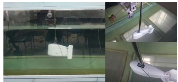
Fig. 16 Partial captive model experiment in circulating water channels
