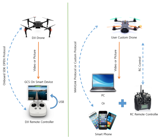
Fig 3. Data Communication of Drone between General GCS
