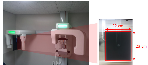
Fig. 2. Experiment for measuring X-ray exposure area (left: setup, right: result).
