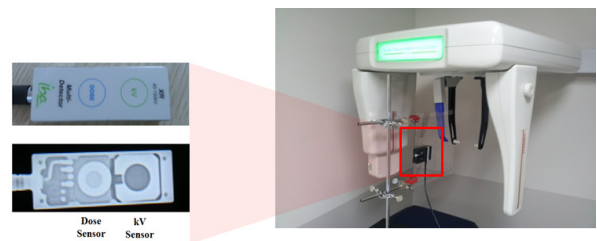
Fig. 3. Setup of experiment for measuring X-ray dose distributions (left: MagicMax dosimeter, right: location of the dosimeter in cephalometric radiography system).
