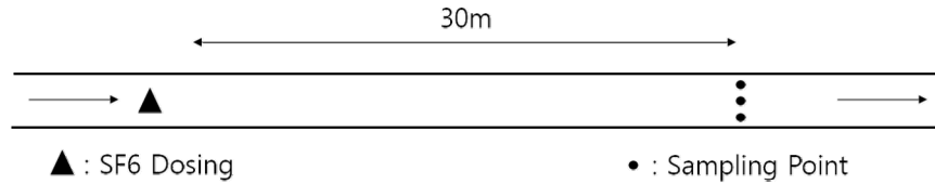
Fig. 2. Diagram of flow measurement by using tracer gas
