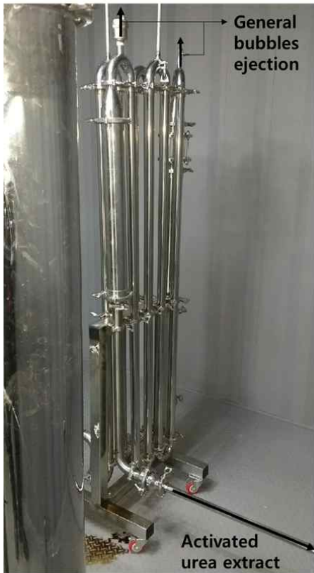
Fig. 5 Activated urea extract pipe
