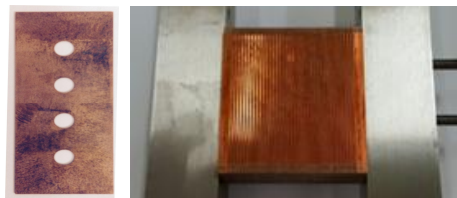
(b) Fixed Cu sheets for the improved tests
