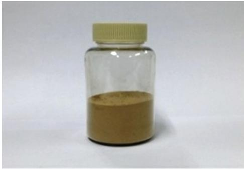
**Fig. 2.** MAP crystals recovered from biological livestock wastewater treatment plant.
