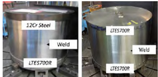
Fig. 5 LTES700R welding test
