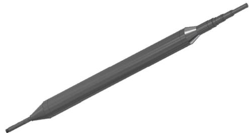
Fig. 8 Shaft of Primary Pump
