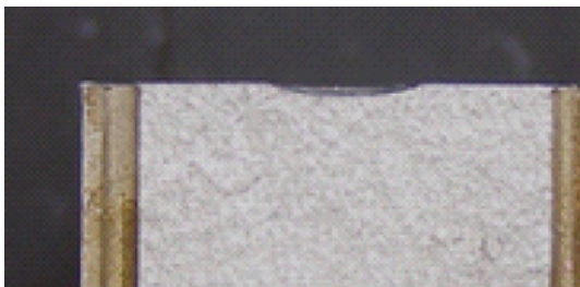
Fig. 2 Fracture surface after the fracture tests ( a/W=0.3 )
