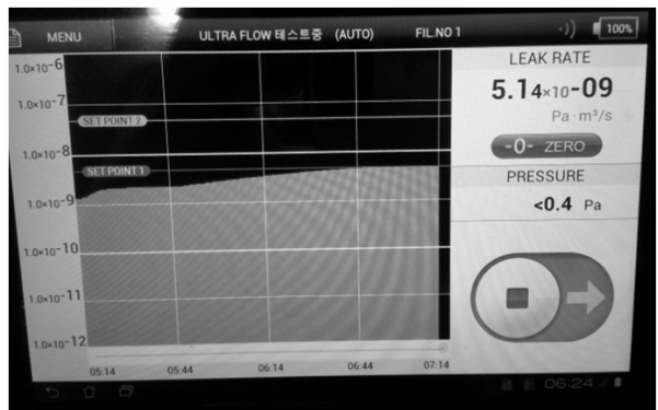
(b) Measured leak rate
