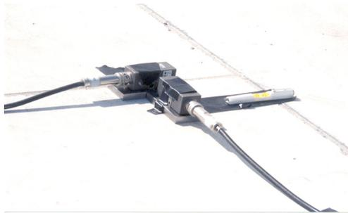
(a) Servo accelerometer installation situation
