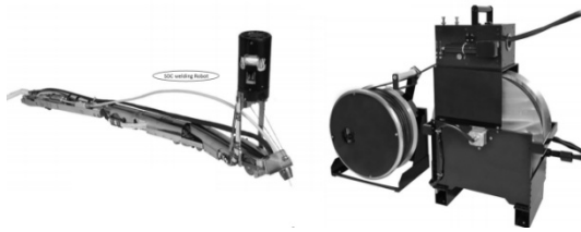
[Figure 21] Diakont welding robot and deployment station with welding rod pusher [18]
