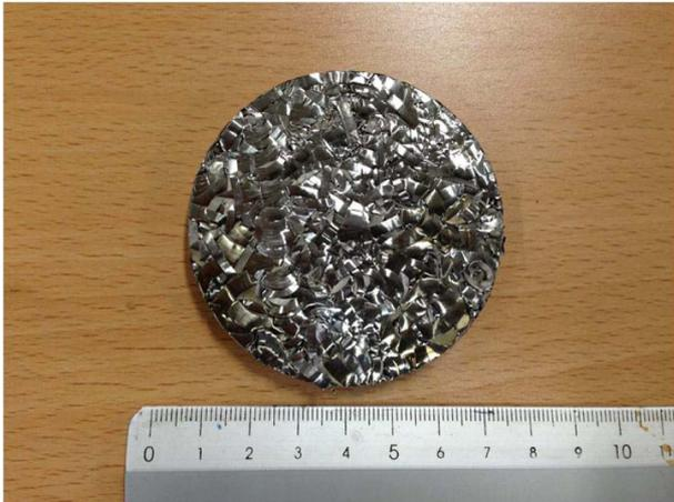
Fig. 1. Scrap compact for arc melting.
