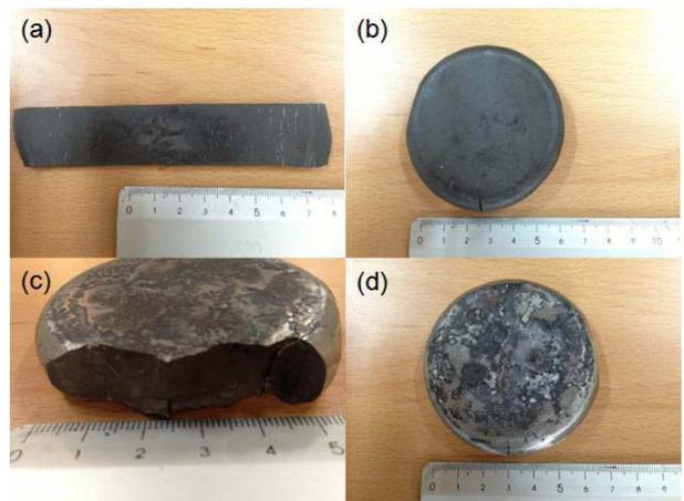
Fig. 3. Photographs of the Zr alloys processed by hot rolling. (a) Zr-1.2Nb-0.2Fe, (b) Zr-1.2Nb-0.3Fe, (c) Zr-1.2Nb-0.28Fe<sub>2</sub>O<sub>3</sub>, (d) Zr-1.2Nb-0.43Fe<sub>2</sub>O<sub>3</sub>.
