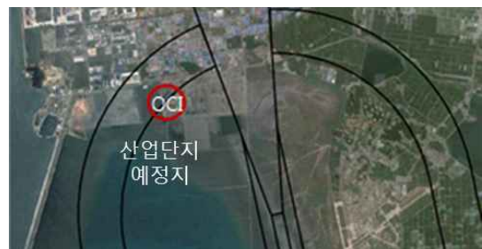
Fig. 6 Critical obstacle vs obstacle limitation surfaces of the 1st case
