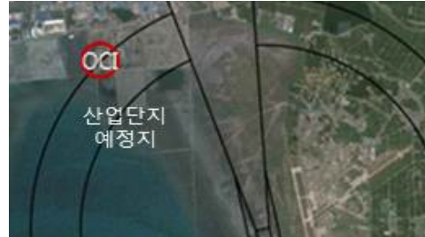
Fig. 8 Obstacle limitation surfaces of staggered runway
