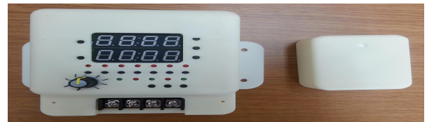
Fig. 6. Full Image of Illuminance Detector and Energy-Efficient Automatic Power Controller of signboard.
