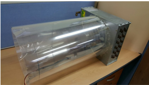
Fig. 1. Photo of experimental FCU (Kim, 2016b).
