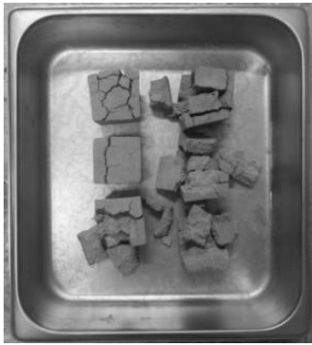
Fig. 9 Cube specimens after thermal cycling for mixtures including CSA(M5 and M6)
