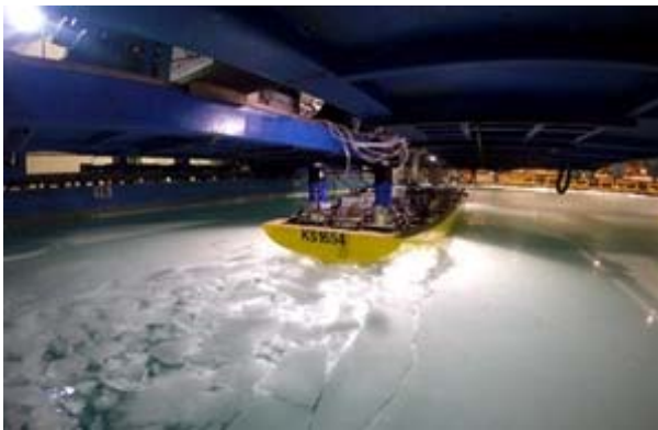
Fig. 2 Model test in level ice condition
