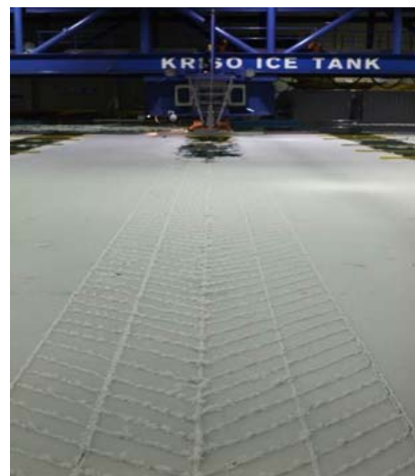
Fig. 1 Pre-sawn ice condition in ice basin
