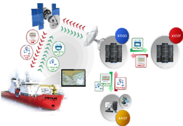
Fig. 1 Conceptual architecture of voyage planning system for Araon
