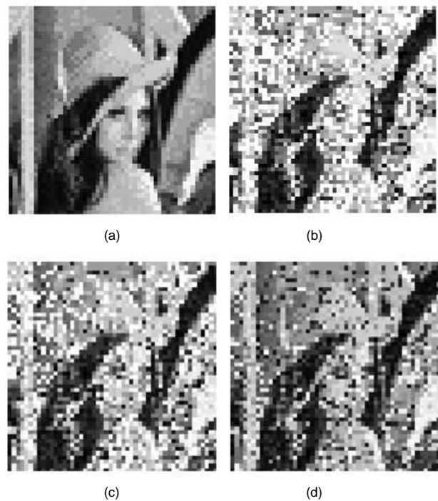
Fig. 8. Experimental results: (a) original, (b) without the equalizer, (c) with real-coefficient equalizers, and (d) with a complex-coefficient equalizer.
