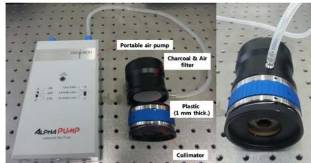
Fig. 10. The airborne dust sampler and collimator.
