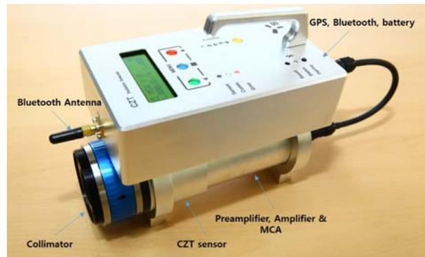
Fig. 9. Developed in-situ gamma-ray spectrometer based on the CZT detector.
