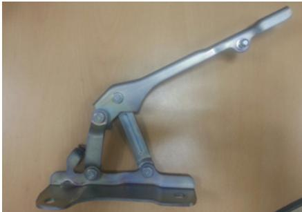
Fig. 1 Hood frame of vehicle
